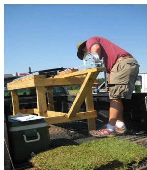
Mechanism used to determine sod strength - a measurement of the force required to tear a piece of sod.
