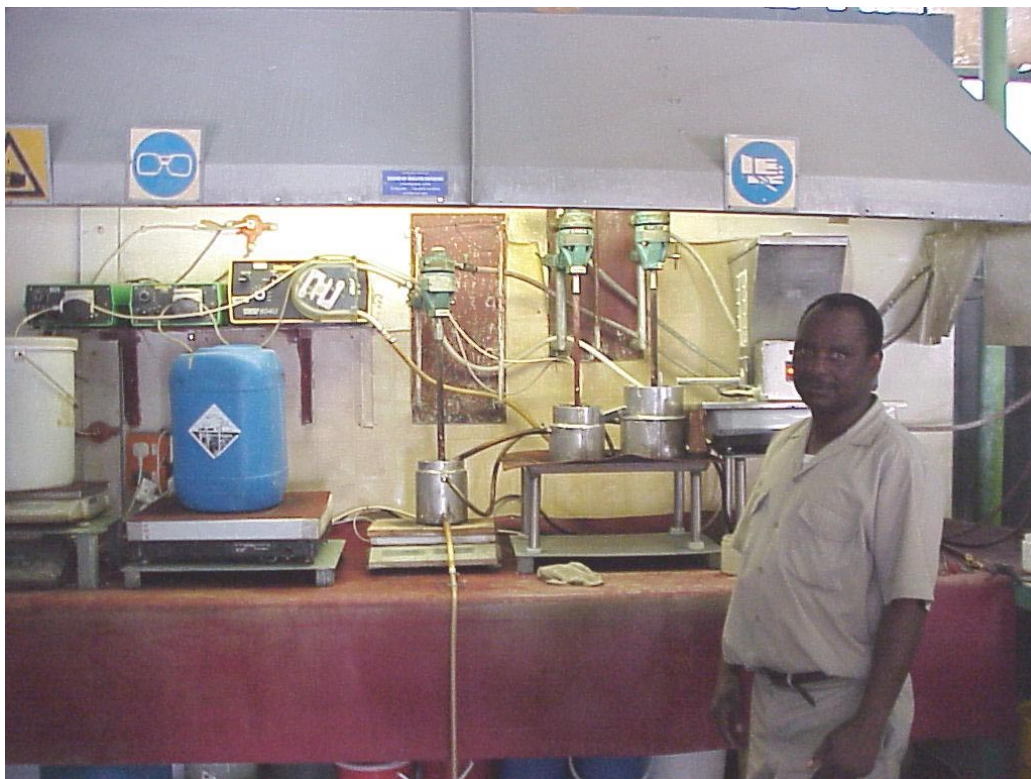
Figure 5. Foskor's phosphoric acid pilot-plant facility showing feed pumps, reactors, rock screw feeder and maturation tank.
