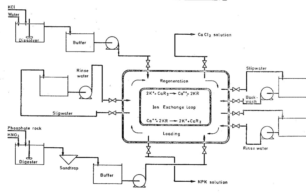
The inlet and outlet places for the liquids are moved stepwise forward in the loop thereby displacing the loading and regenerating sections around the loop.
