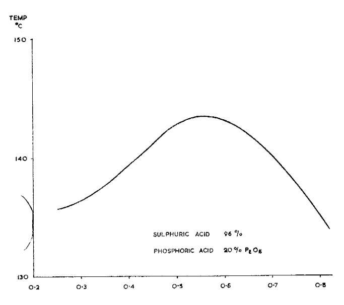
RATIO LBS/HR RECYCLED PHOSPHORIC ACID PER LB/HR SULPHURIC ACID
